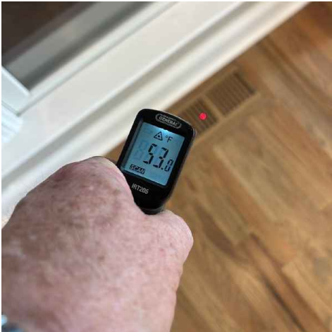
First floor AC temp
